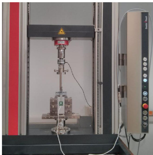
Figure 2: Experimental setup for the TPB test.
