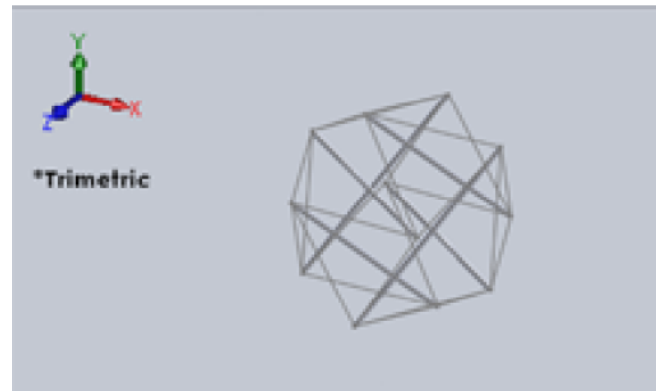
Figure 1: Classical cell tensegrity structure.
