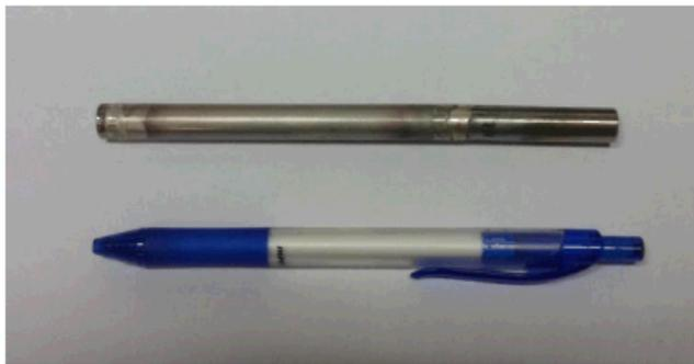
Figure 2: Dense self-supported Pd-Ag membrane.
