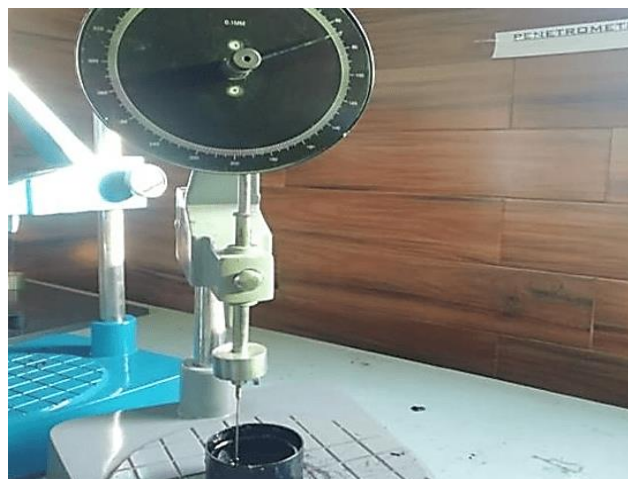
Figure 3: Penetration test apparatus in the laboratory
