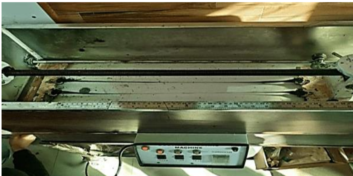
Figure 5: Ductility test apparatus in the laboratory
