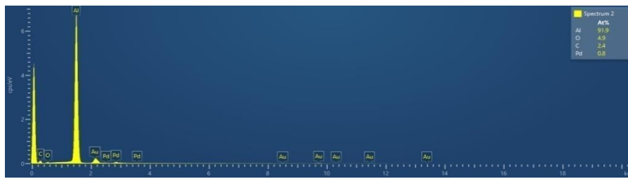
Fig.7. EDS of AL+2%wt RGO by the wet method.
