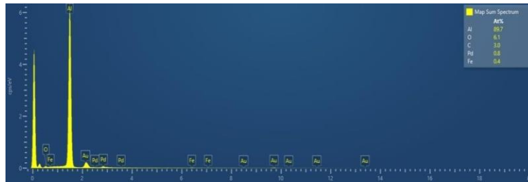
Fig.9. EDS spectra of AL+2%wt graphene by ball milling.
