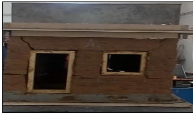
Figure 6: Collapse occurs of model A1
