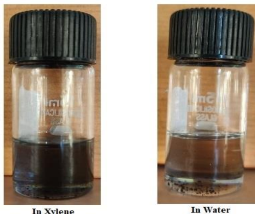
Figure 3 Dispersion of additive in water and xylene
