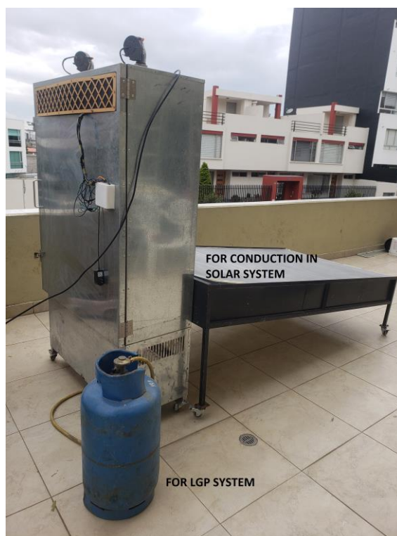
Figure 4. Solar-gas hybrid dehydrator machine on site ready for dehydration.
