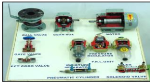
Model Cut Sections - Mechanical Equipment
