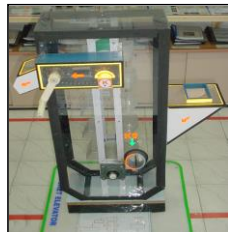
Models Mechanical - Bucket Elevator
