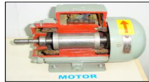
Cut Section Electrical - Motor
