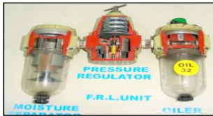
Cut Section Mechanical - FRL Unit
