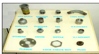
Model Mechanical - Pipe Fittings
