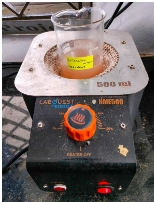
Figure 1: Boiling of Guilandina bonduc seed extract using heating mantle.
