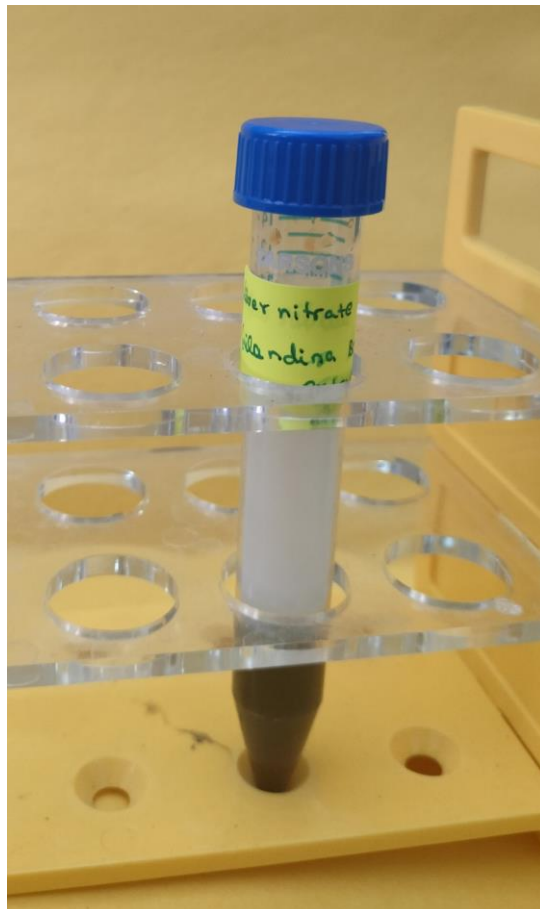
Figure 4: Collected silver nanoparticles after centrifugation
