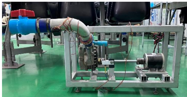
Figure 6. Practical Implementation of the Speed Control System Structure
