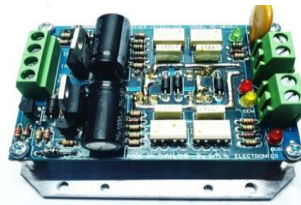
Figure 3. Motor Drive Board for 24V 80A DC Electric Motor
