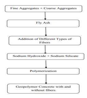
Figure 1: Preparation of Geopolymer Concrete
