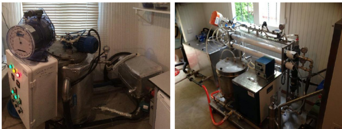
Figure 1: The experimental setup of a) pilot scale biogas system and b) pilot scale membrane filtration system.
