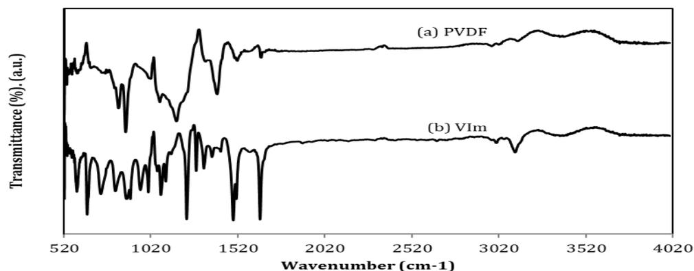
**Figure 5.** FTIR spectrum of (a) PVDF and (b) VIm sample showing transmittance (T%) as a function of wavenumber ( $\text{cm}^{-1}$ ) for the range 4020-520  $\text{cm}^{-1}$
