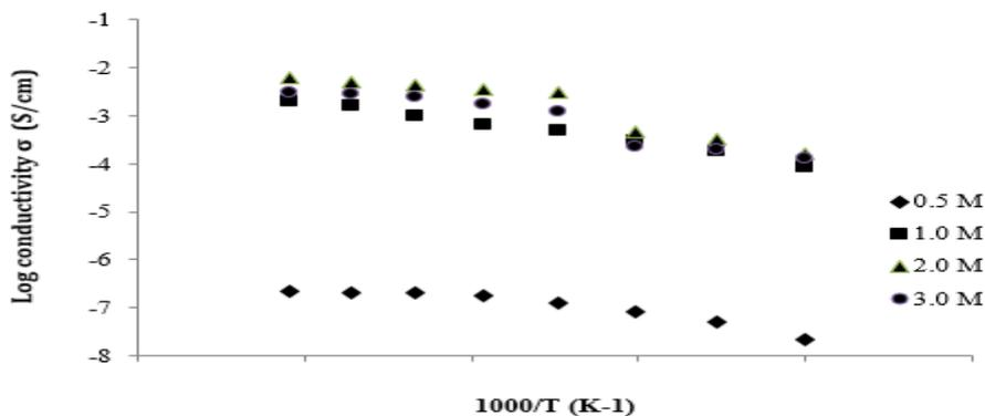
**Figure 8.** The conductivity study at different concentrations of VIm grafting onto PVDF backbone at 60 kGy of absorbed dosed (c) combination all concentration
