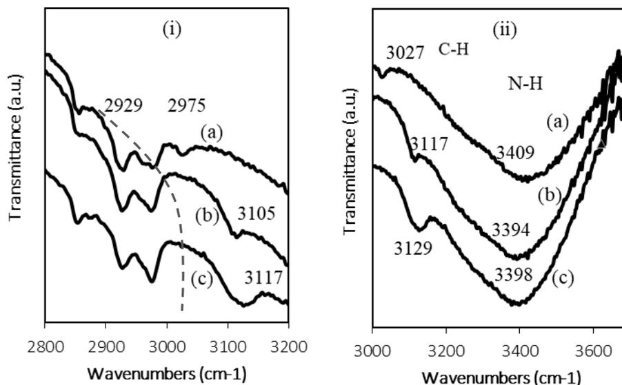
**Figure 7.** FTIR spectra of (a) pristine PVDF, (b) PVDF-g-P1VIm, and (c) protonated PVDF-g-P1VIm in a region between (i) 2800 and 3200 & (ii) 3000 and 3700  $\text{cm}^{-1}$
