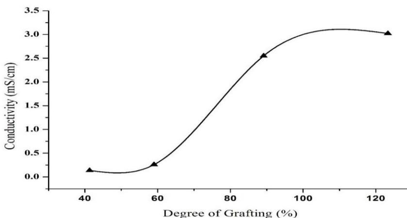
**Figure 10.** Correlation degree of grafting and conductivity
