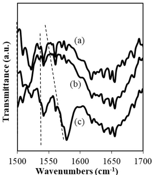
**Figure 6.** FTIR spectra of (a) pristine PVDF, (b) PVDF-g-P1VIm, and (c) protonated PVDF-g-P1VIm in a region between 1500 and 1700  $\text{cm}^{-1}$ .
