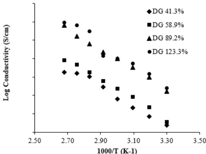
**Figure 9.** Proton conductivity of protonated PVDF-g-P1VIm membrane at varying DG is temperature dependent.
