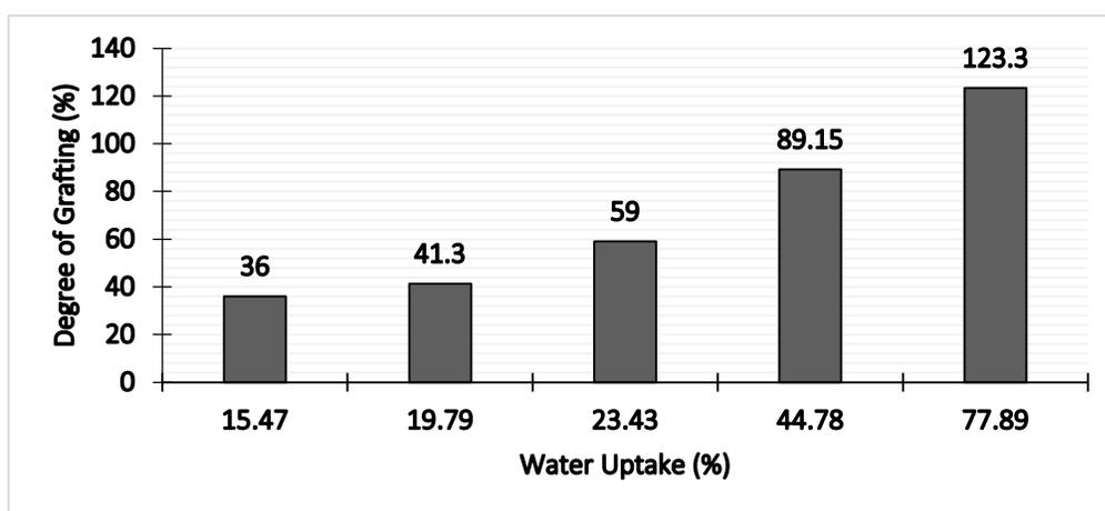
Figure 3. Effect of water uptake on the various degree of grafting for protonated PVDF-g-P1VIm membranes
