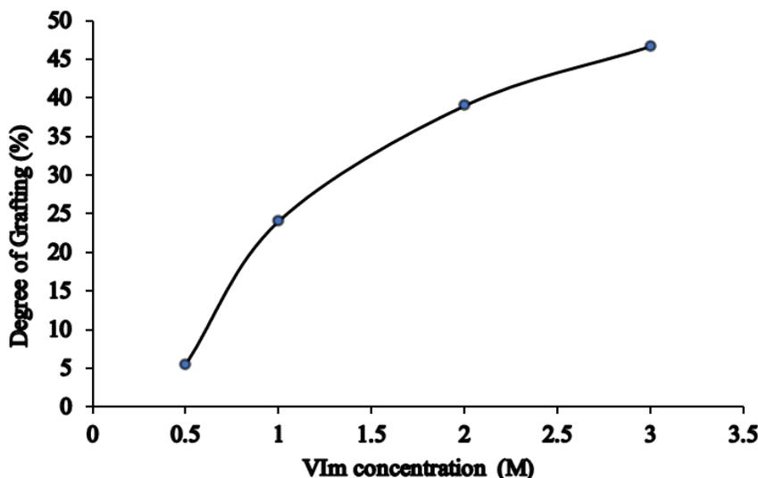
**Figure 1.** Effect of VIm concentration on grafting yield of PVDF backbone at 60 kGy of absorbed dose.
