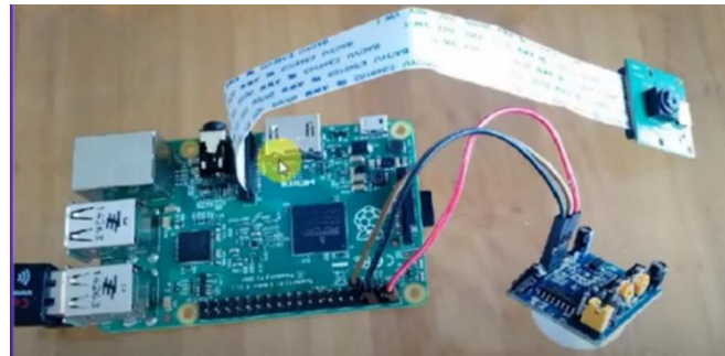
Fig. 8 . PIR sensor with camera
