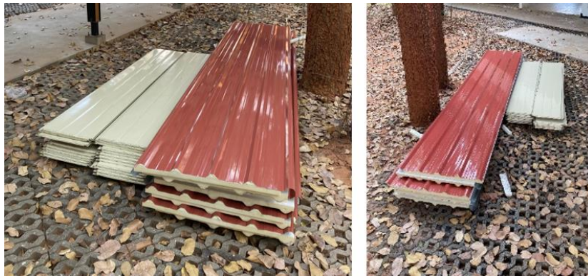
Fig. 7. The metal sheet roof and wall panel
