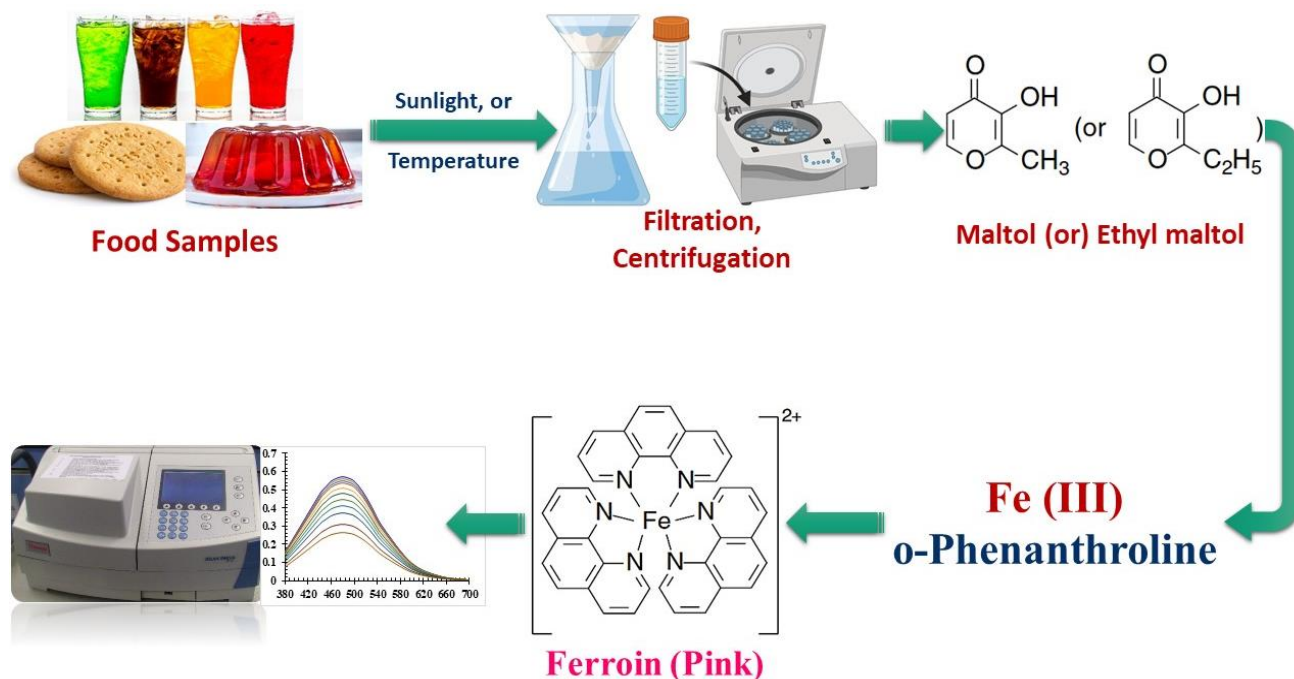
Figure 1. Illustration of maltol and ethyl maltol determination steps.
