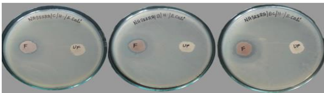
Figure 7. Antibacterial activity of Latana camara L. extract finished fabrics against Escherichia coli
