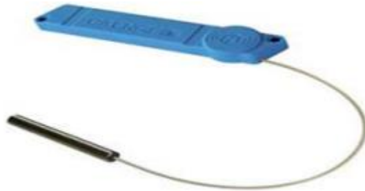
Figure 2.4: A picture of a UHF semi-passive RFID tag with a temperature probe (Source: Veryfields.net)
