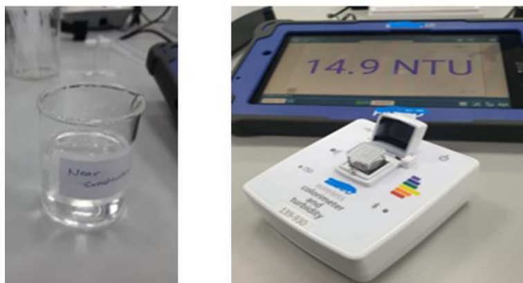
Figure 1. Experimental testing of a water sample, and Turbidimeter
