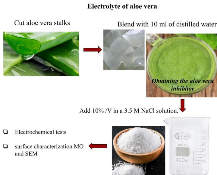
Figure 1.- Sequence of the elaboration of the electrolyte 1 and 2 used for the electrochemical and immersion tests.
