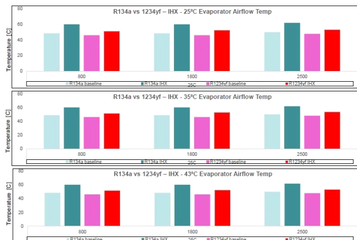
Figure 6: Compressor Discharge Temperature
