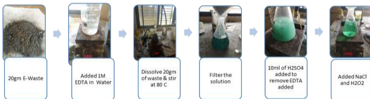
Figure 5. Experimental set up for preparing Electrolyte
