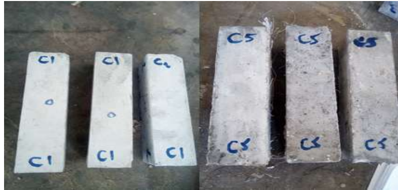
Figure 5. Specimens of (traditional plaster + palm fibres)
