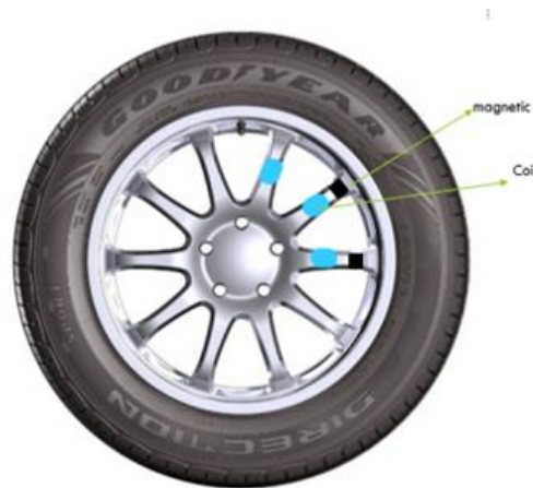
Figure 1. Schematic drawing illustrating placement of magnetic and coils in Spokes
