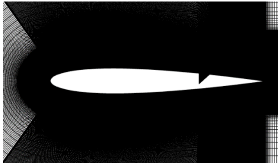
Fig. 5. The meshing around the cavity and airfoil.
