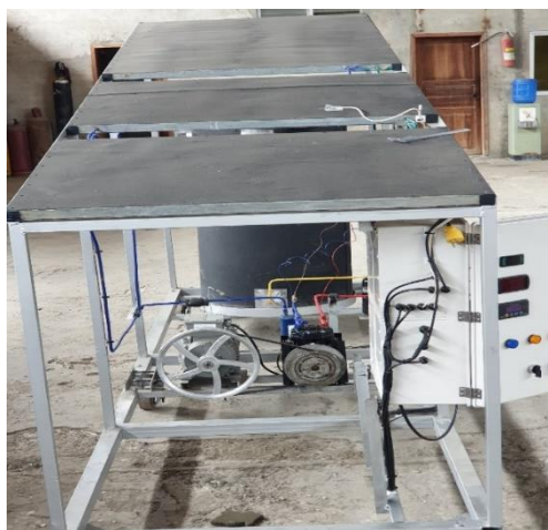
Figure 2. Frontal view of a direct expansion solar assisted heat pump
