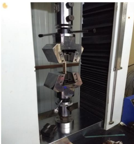
Figure 3 Tensile Testing of composite in Universal Testing Machine
