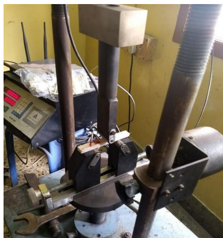
Figure 4 Flexural testing with 3 point bend test fixture
