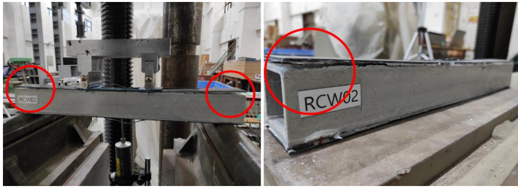
Fig. 2. Destruction of the adhesive part of the specimen
