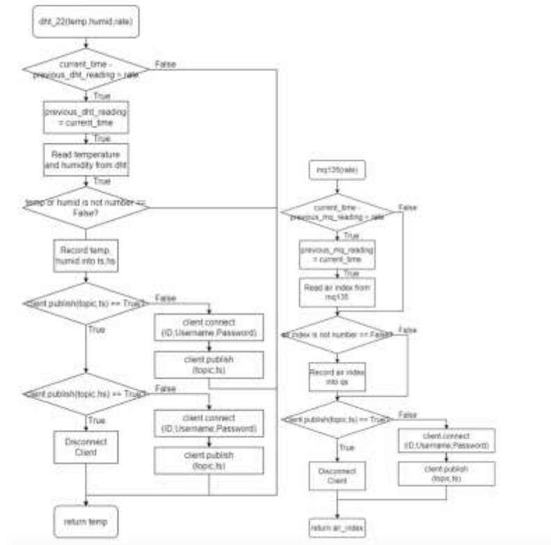
Figure 4: Program flowchart of dht_22 and mq135 function for Smart Shelf
