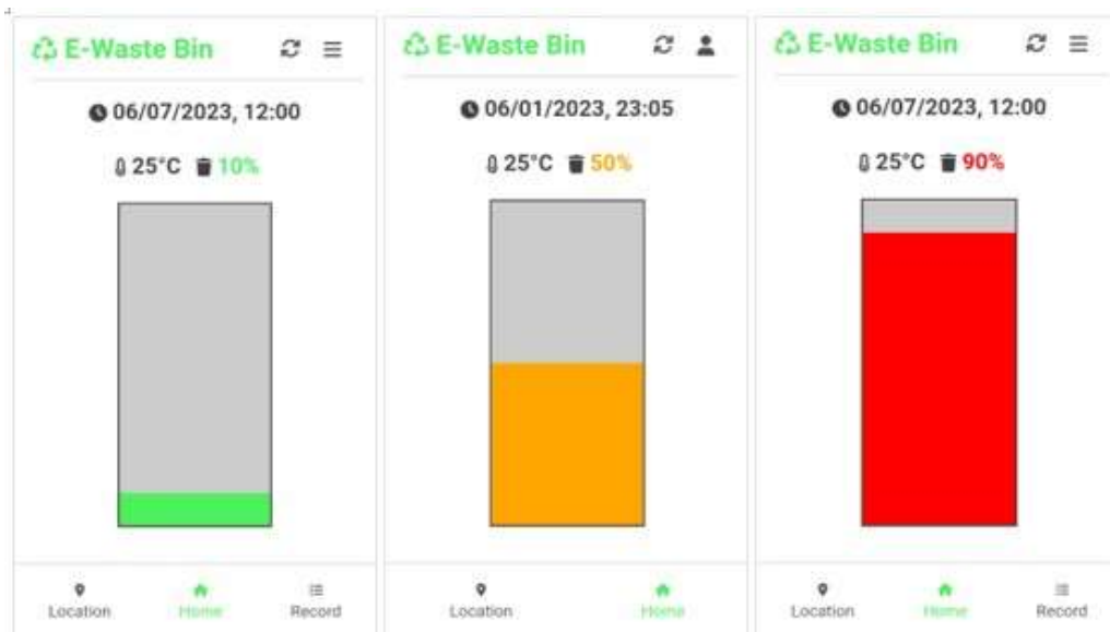
Fig. 6: Home Screen with Different Bin Fill Level
