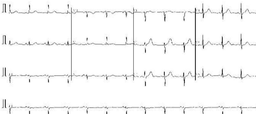
Fig. 5: The results of removal of gridlines after implementation of image convolution.
