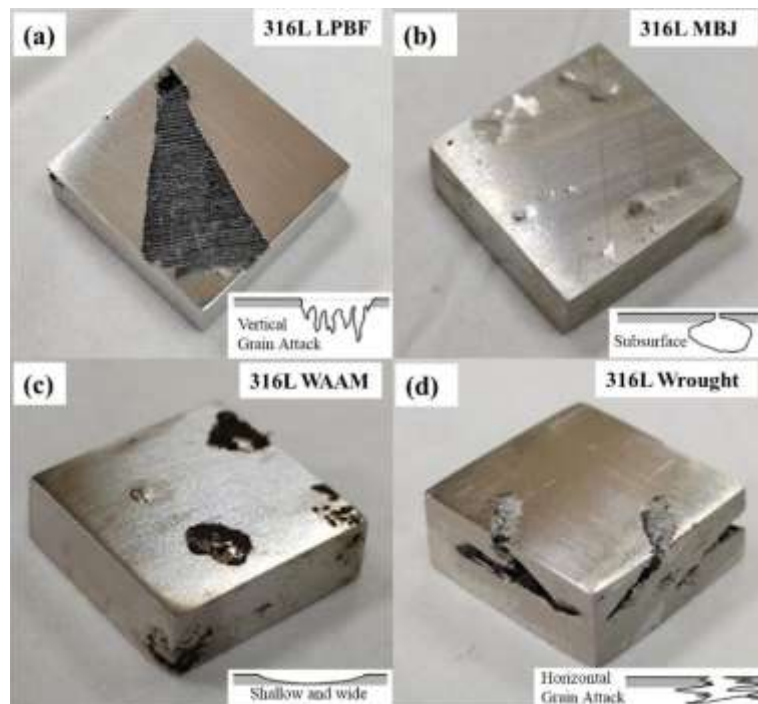
Fig. 8: 316L stainless steel corrosion characteristic of (a) LPBF, (b) MBJ, (c) WAAM, and (d) Wrought
