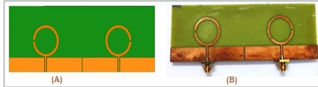
Fig 3 Antenna array with 1 x 2 configuration as a (A) Simulated design (B) Fabricated design.
