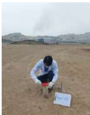
FIGURE 1: SAMPLING OF CONTAMINATED SOIL WITH LEAD
