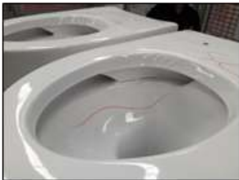
Figure 2. Cracking Defect of a Sanitary Ware
