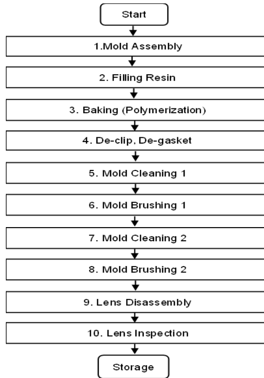
Figure 2. Convex Lens Production Process.
