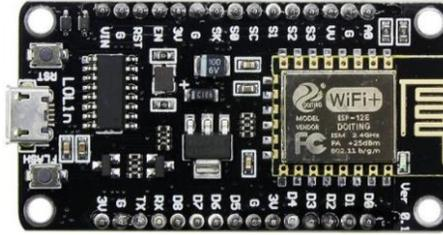
**Figure 5.** Kit RF Transceiver for Wifi ESP8266 NodeMCU Lua V3 CH340.
