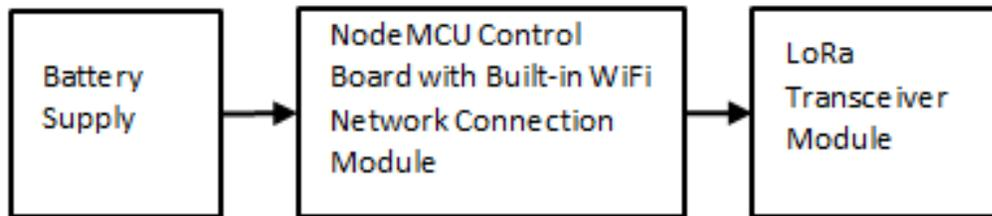
Figure 4. Block Diagram of the Communication Circuit of a Gateway.
