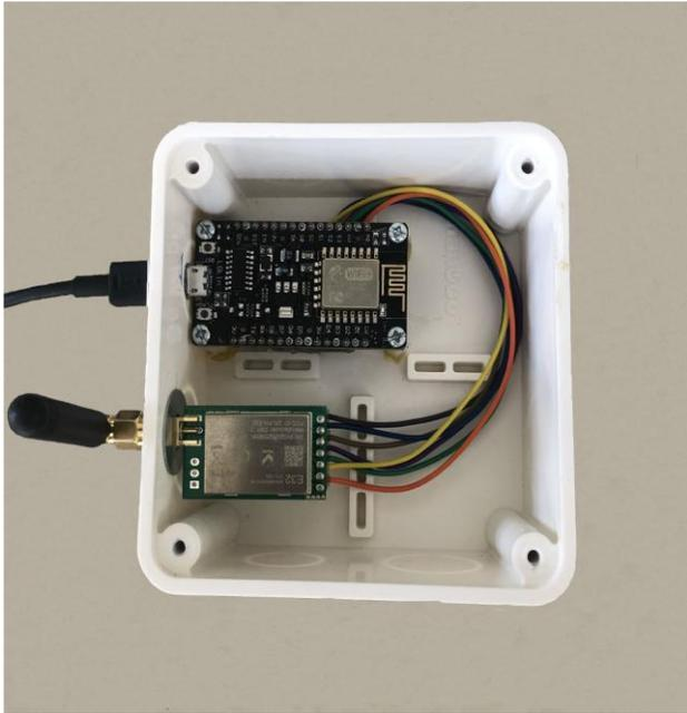
**Figure 12** includes: Control board with integrated WiFi Plus (WiFi +) network connection module ESP8266 NodeMCU Lua CH340, RF transceiver module SX1278 Lora E32.
