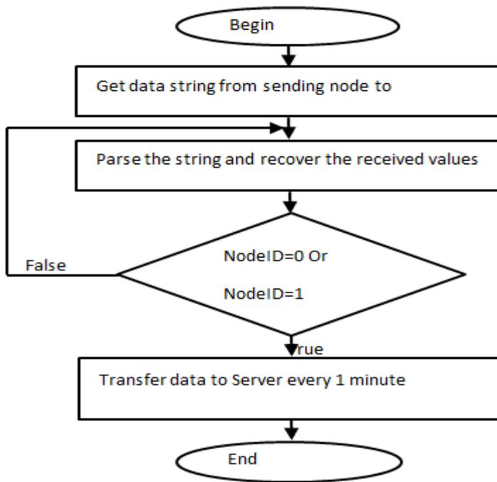
**Figure 6**, including 03 main steps as follows: Step 1 - Initialize and configure the Setup() function: Initialize the UART, configure the signal pins, configure the WiFi connection, configure the connection to the Server. Step 2 - Build the loop() function: parse the string and recover the values received from node. Step 3 - Build the function PostDataToServer(): to transmit to the Server the sensor values that have been analyzed and recovered from the loop() function.
