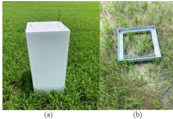
Figure 10. (a) Chamber Body, (b) Chamber Base.
