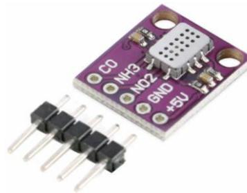
**Figure 5.** MICS-6814 Air Quality CO NO<sub>2</sub> NH<sub>3</sub> Nitrogen Carbon Gas Sensor Module For Arduino.
