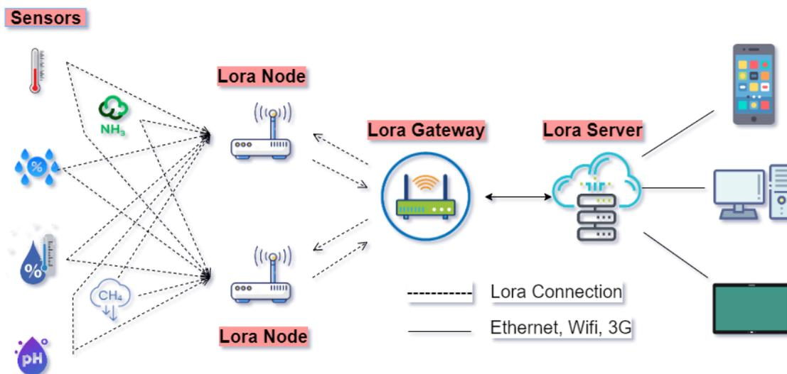
Figure 1. The Overview of our Proposed LoRa Wireless Sensor Network Model in An Giang, Vietnam.
