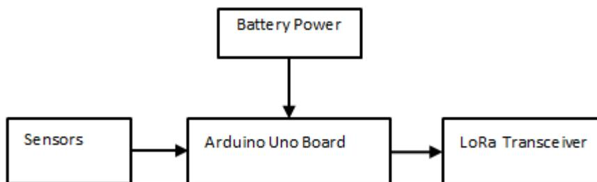
Figure 2. Block Diagram of a LoRa Node.
