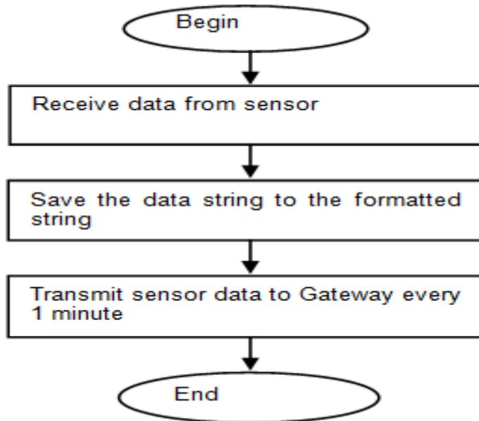
Figure 3. Flowchart of Signal Processing Algorithm at a Lora Node.
