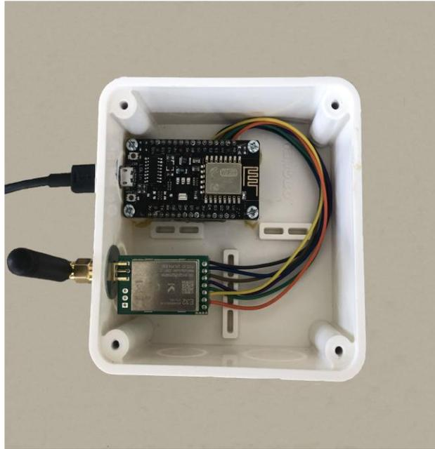
**Figure 12.** The Actual Circuit of Lora Gateway.
