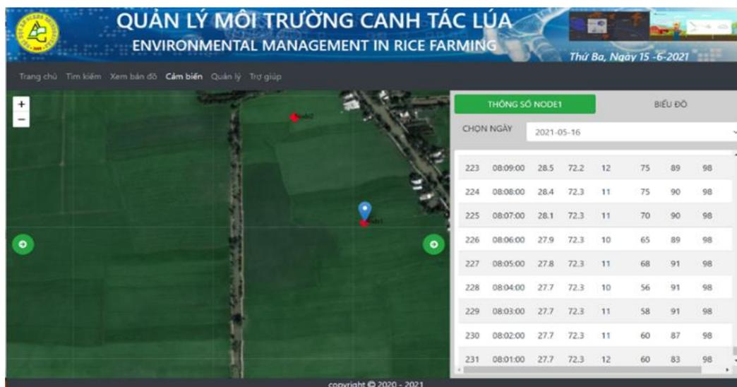
Figure 20. The WebGIS System Displays the Value of the LoRa Nodes.
