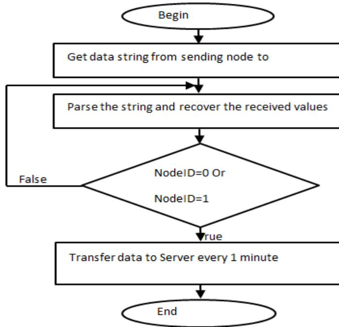
Figure 6. Flowchart of Processing Algorithm for Lora Gateway.
