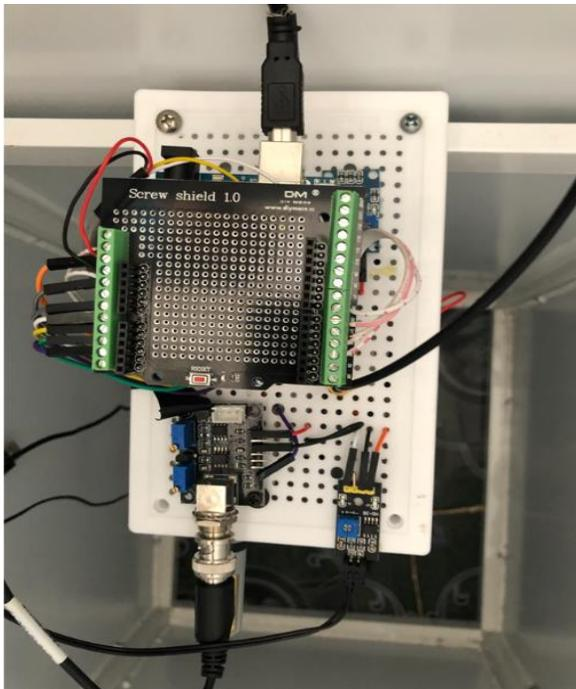
**Figure 11** includes: Arduino Uno R3 controller board, SX1278 Lora E32 RF transceiver module, 12V DC battery power, sensors. Lora Gateway has the function of collecting data from Nodes and simultaneously transmitting it to the server. The actual circuit of Lora Gateway as shown in
