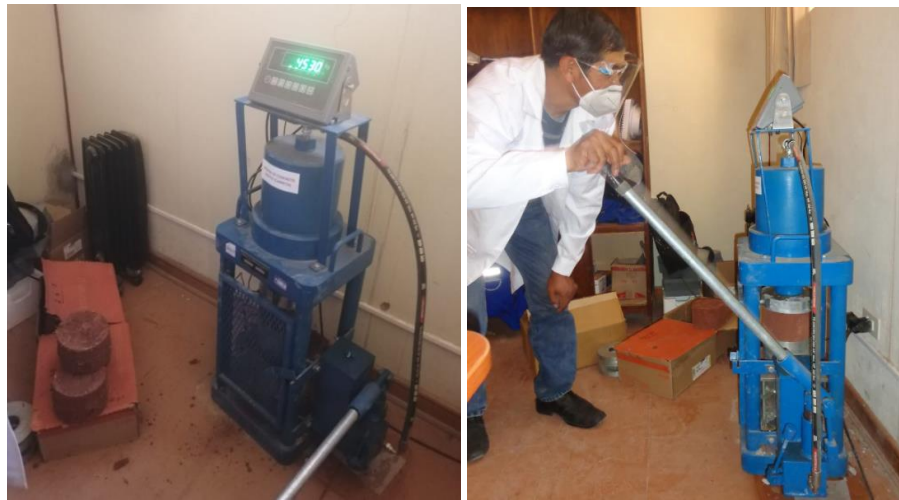
Figure 3. Hydraulic press for compressive strength testing.
