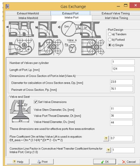
Figure 5. Diesel-RK software gas exchange parameters – Intake port
