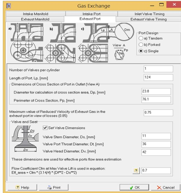
Figure 4. Diesel-RK software gas exchange parameters – Exhaust port
