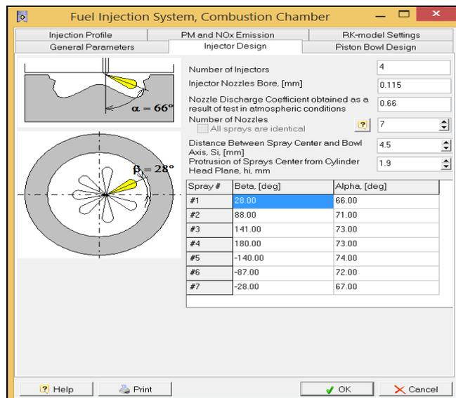
**Figure 3.** Fuel Injection Nozzle Details in Diesel-RK Software
