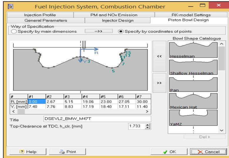
**Figure 2.** Piston bowl defined in the Diesel-RK software.
