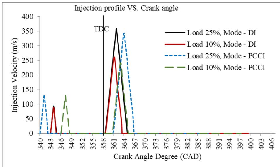
Figure 6. Fuel injection velocity at different crank angles
