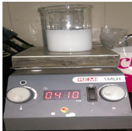
Figure 2: \text{TiO}_2 and CAP solution on a magnetic stirrer at 400rpm.
