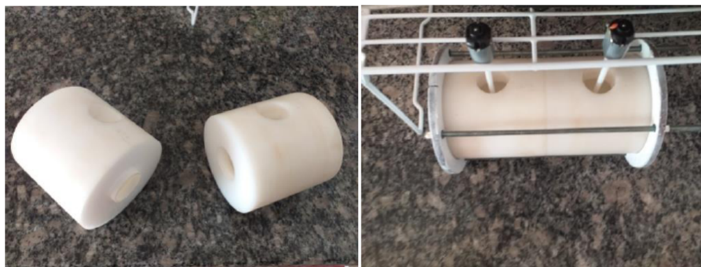
Figure 2: Membrane reactor used in separation/recovery of phenols mixture.
