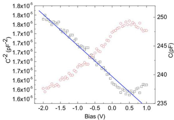
**Figure 9:** Capacitance (C)-Voltage (V) characteristics of the Fe/p-Si heterojunction.
