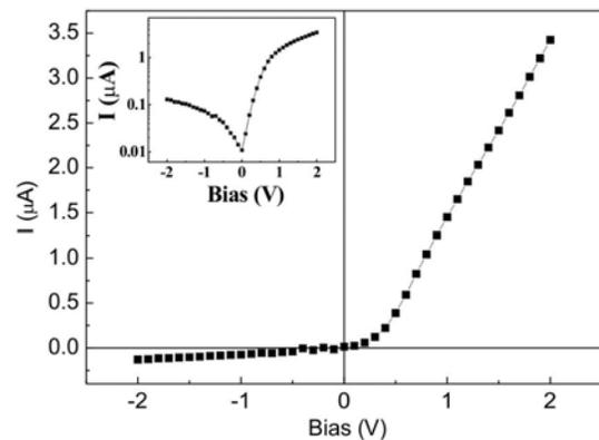
**Figure 7:** Current (I)-voltage (V) characteristics of Fe/p-Si, measured at 300 K. In the inset shows the semi-log I-V characteristics representing the Schottky behavior.
