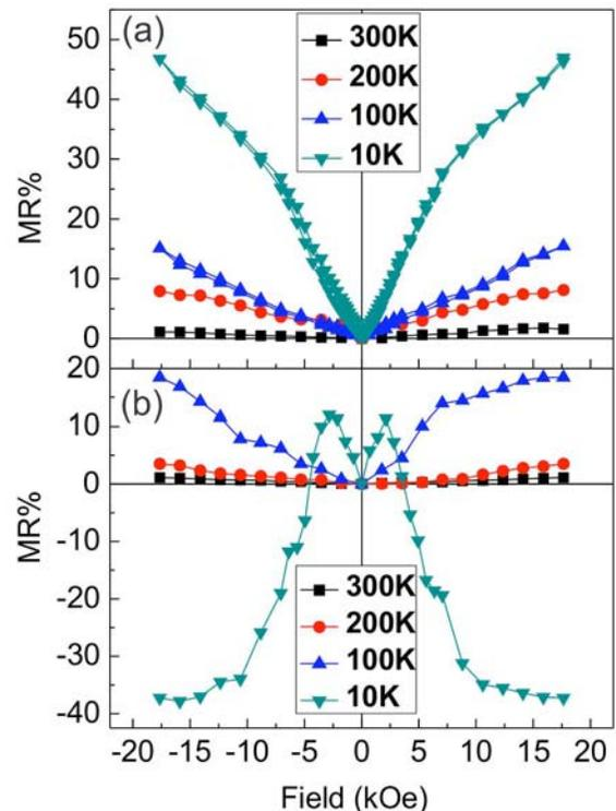
**Figure 5:** Magnetoresistance (MR) of Fe-film measured on application of field ( $H$ ), (a) perpendicular and (b) parallel, to the direction of current as well as the plane of the film.
