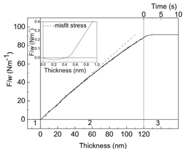
**Figure 2:** Force per unit film width  $F/w$  evolving as a function of mean film thickness and time during and after the growth of Fe on the Si substrate; the inset shows the zoomed image of the force curve at lower thickness. The dashed line represents the constant strain in the film during initial stage of the film growth.
