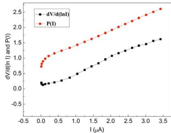
**Figure 8:**  $dV/d(\ln I)$  and  $P(I)$  versus  $I$  plot of the Fe/p-Si heterojunction.
