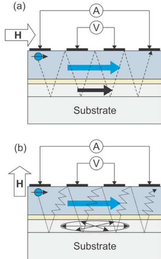
**Figure 6:** Schematic representation of the CIP mode of the measurement of magnetoresistance of the Fe film with magnetic field applied (a) in-plane and (b) out of plane, to the film.
