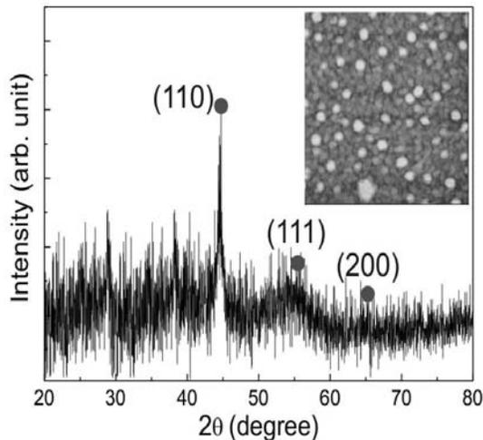
**Figure 1:** XRD measurement of Fe film (120 nm). The inset shows  $1\mu\text{m} \times 1\mu\text{m}$  AFM image of the surface of the Fe film.
