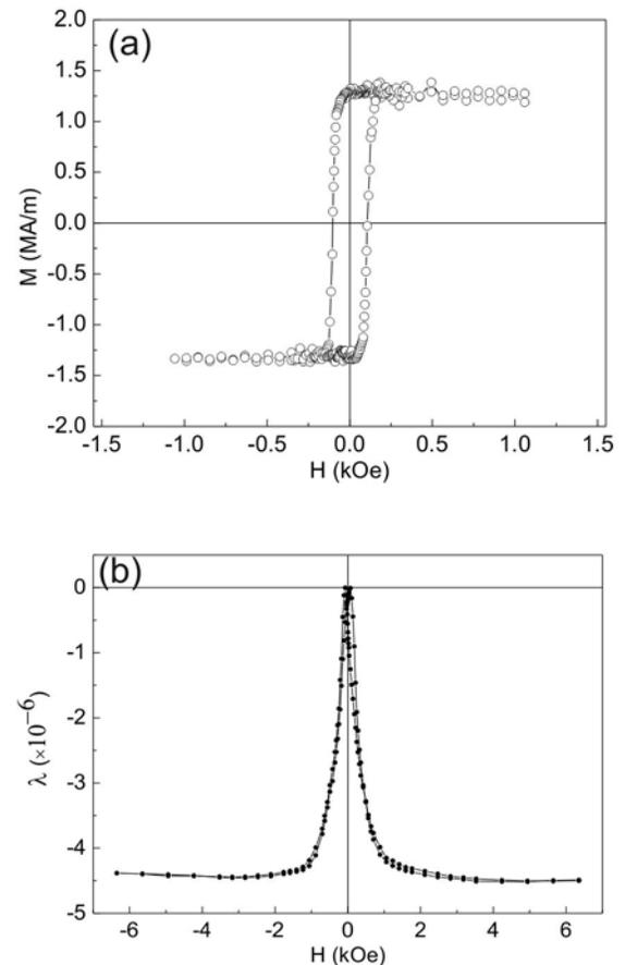
**Figure 3.** (a) magnetization as a function of applied field at room temperature for Fe film; and (b) variation of linear magnetostriction with field applied along the length of the film, measured at room temperature.
