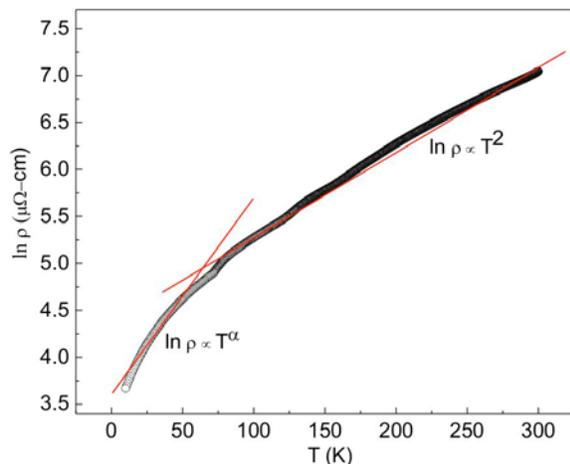
**Figure 4:** Variation of resistivity with temperature of the Fe-film.
