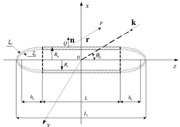
**Figure 1:** Elastic non-analytical shell, compiled from finite cylindrical shell with spheroidal shells on the ends.
