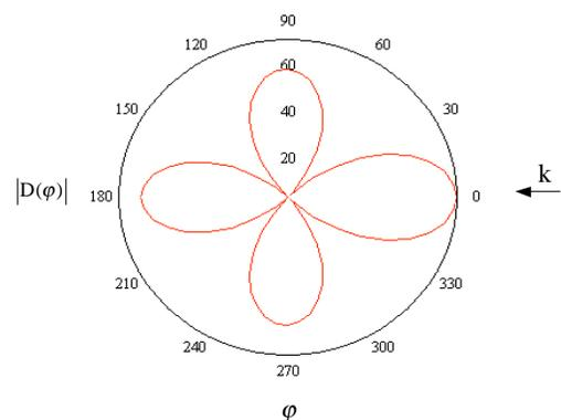
Figure 5: Module of angular characteristic of scattering  $|D(\varphi)|$  for  $ka = 0,523, \theta_0 = 90^\circ$ .
