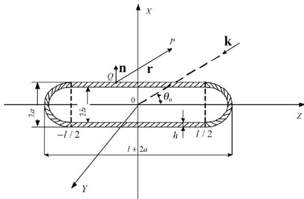
Figure 4: Elastic non-analytical shell, compiled from finite cylindrical shell with hemispheres on the ends.
