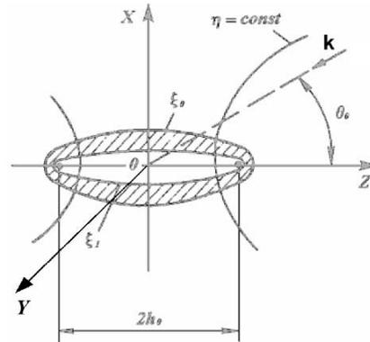
Figure 3: Elastic spheroidal shell.
