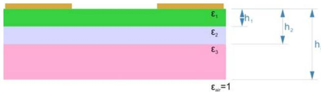
**Figure 3:** The cross-section of two adjacent fingers in IDEs with three-layered structure.
